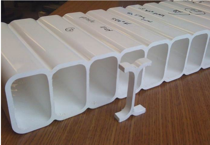
FIGURE 1. EXTRUSION PROFILE AND THE WEB KNIT-LINE SAMPLE AS CUT FROM THE EXTRUSION.
