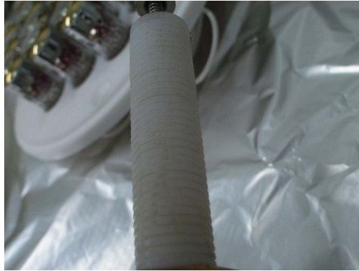
Figure 40: Detail of the carbon tracks produced in the polyethylene of the cathode feed-through during the tests in NEXT-DEMO.
