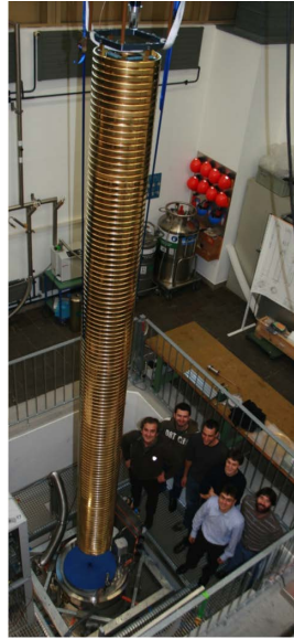
Figure 13: TPC of the ARGONTUBE at LHEP Bern. Gold plated field shaping rings to reduce high voltage breakdowns cover 5 m drift length.
