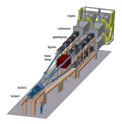
Figure 2: The Super-Beam beam transport and distribution system.
