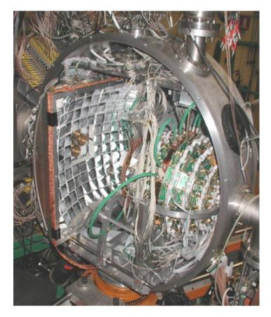
Figure 15: The  $8\pi LP$  experiment used for measurement of the <sup>7</sup>Li(d,p)<sup>8</sup>Li cross-section.
