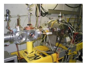
Figure 16: The prototype ion collection device constructed for Beta Beam studies.
