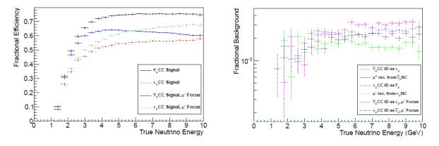
Figure 20: Performance of the MIND detector. (Left) The efficiency for detecting the muon signal events. (Right) The fractional backgrounds.
