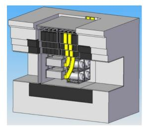
Figure 6: Conceptual design of the section of the target station for the 4 targets and horn systems. The beam enters from the left. The horn pulsing circuits will be mounted on top of the shielding, so the strip lines exit vertically.
