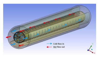
Figure 4: Proposed pebble bed target for the Super Beam.
