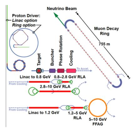
Figure 12: Updated layout for a Neutrino Factory for 10 GeV operation, with only one decay ring. The two options for muon acceleration are shown.
