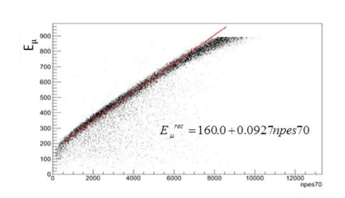
Figure 23: Performance of the MEMPHYS detector. The reconstructed energy of a muon from a neutrino interaction is compared with the real energy, as a function of the number of photoelectrons detected.
