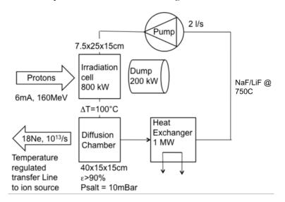
Figure 17: A NaF molten salt loop for the production of <sup>18</sup>Ne ions.
