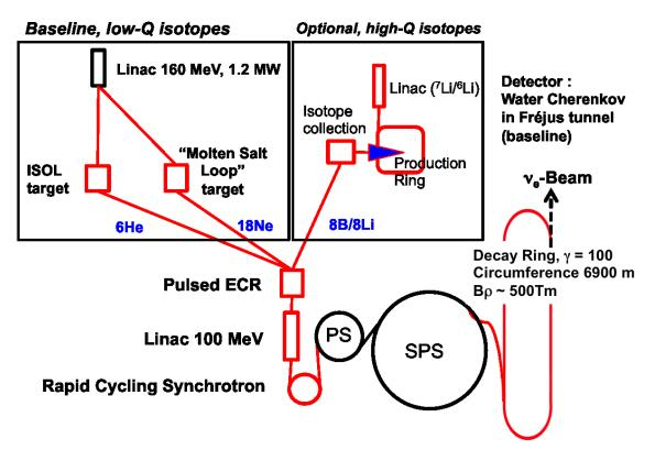
Figure 14: Layout of the CERN Beta Beam.
