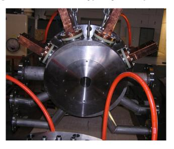
Figure 18: The SEISM 60 GHz ECR source prototype.
