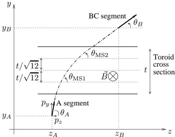
FIG. 4: Scheme of the local track fitting method. In this example, a muon is crossing the central top part of the muon system. Thus the coordinate measured by the segment is  $z$ , the deviation plane is  $(z, y)$ , and the magnetic field ( $\vec{B}$ ) is oriented along the  $x$ -axis. See text for details.
