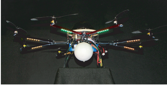
Figure 1: The Octocopter with the light source suspended below it. Green LEDs indicate the forward direction.
