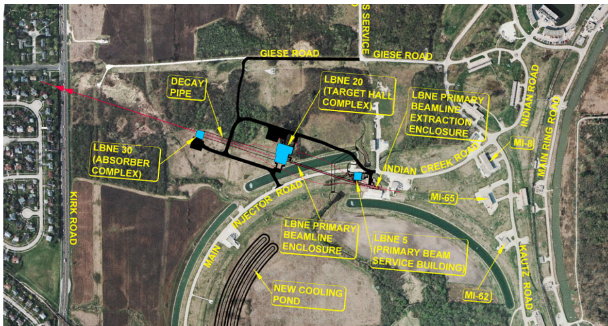
Figure 3-9: Plan view of the overall Near Site Project layout showing the LBNE Beamline extraction point from the Main Injector, the primary beamline, target hall, decay pipe and absorber.
