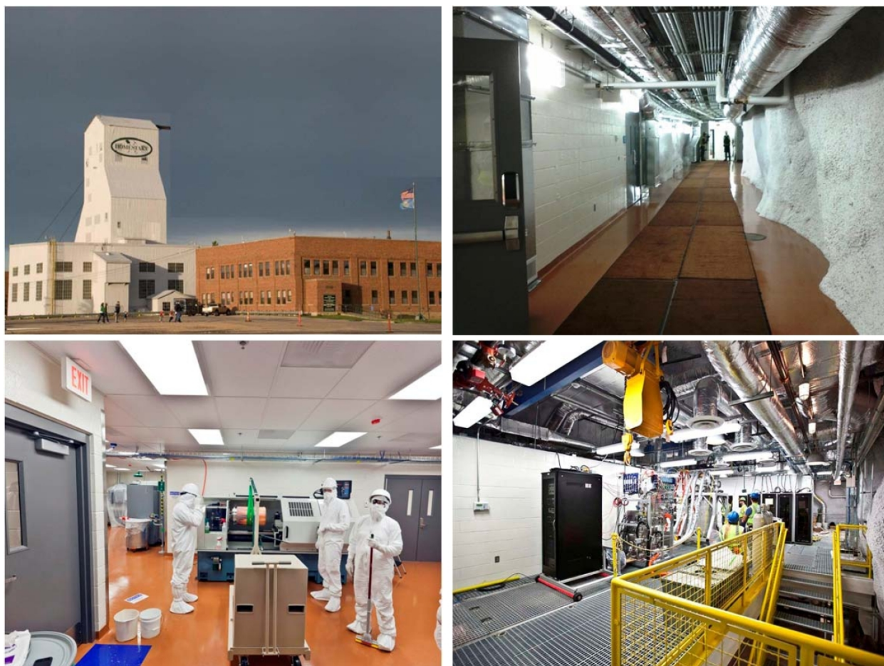
Figure 3-3: Sanford Underground Research Facility: Administration building and Yates shaft headframe (top left); corridor at 4850 ft (1480m) depth leading to clean rooms and experimental halls (top right); billet of radiopure electroformed copper for the Majorana Demonstrator experiment being placed on a lathe in a clean room at 4850 ft depth (bottom left); LUX experiment at 4850 ft depth (bottom) right.
