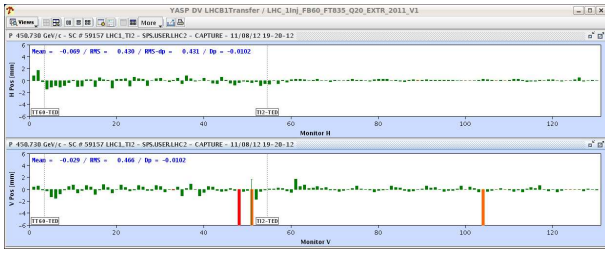
Figure 2: Trajectory for the TI2 transfer line. The top plot shows the difference between the horizontal trajectory measured with the Q20 optics and the golden trajectory. The bottom plot shows the same for the vertical plane.
