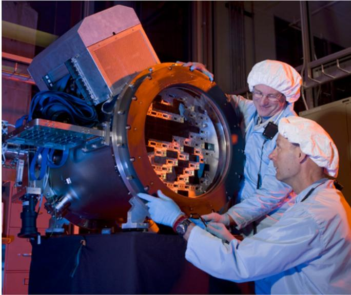
Figure 3. The prototype imager with engineering grade CCDs in May 2009.
