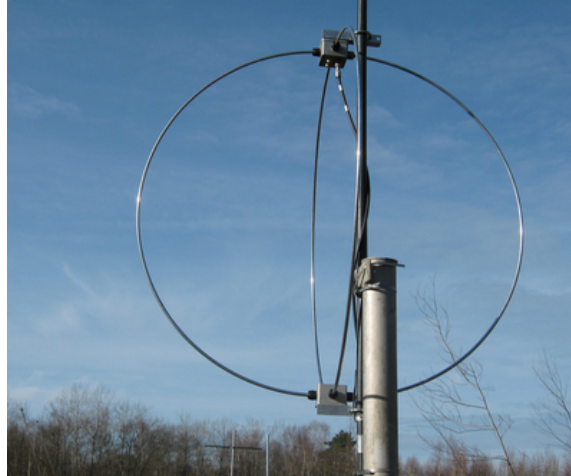
Figure 3: The Salla antenna during test measurements at the Nançay Radio Observatory. The Salla realizes a Beverage antenna as a dipole loop of 1.2 m diameter. The antenna is read out at the top with an LNA. The amplified signal is guided through the antenna structure to the bottom.
