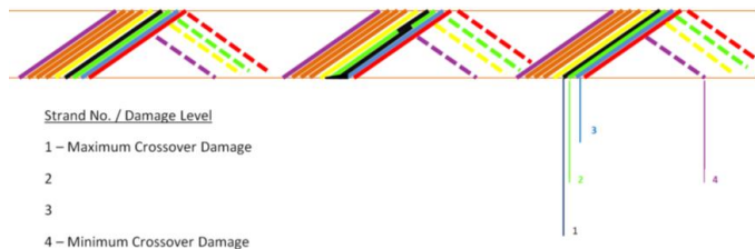
Fig. 20. Schematic of cross-over layout in cable ID 1. Strands No. 1 and No. 2 crossed at an edge and re-crossed within the following half-pitch length.
