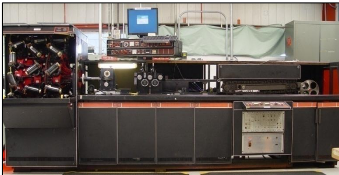
Fig. 1. FNAL compact cabling machine with 42 spools and electronic synchronization for control of cable lay angle.
