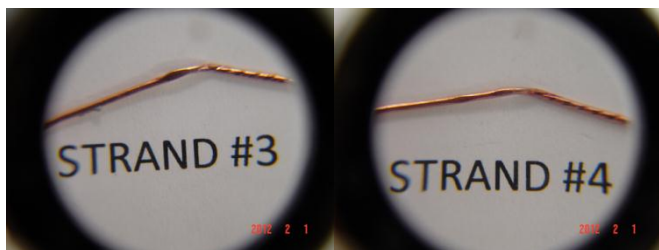
Fig. 23. Picture of area in strand No. 3 closest to first damaged area (left), and picture of area in strand No. 4 closest to second damaged area (right).
