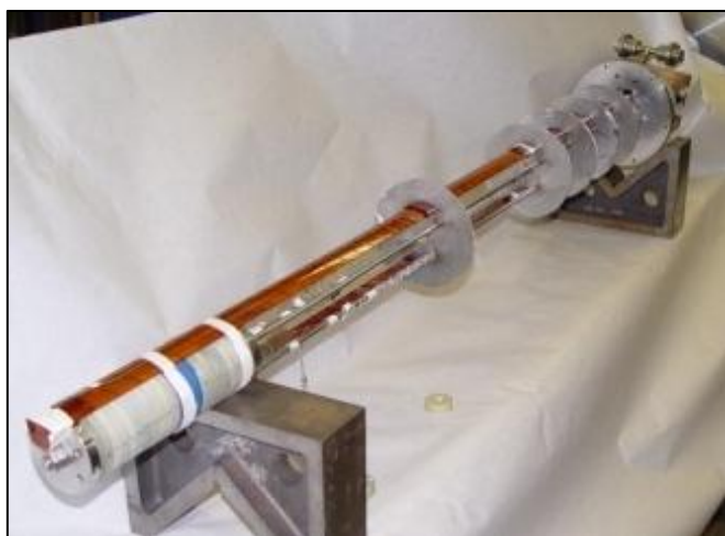
Fig. 7. Modular Insert Test Facility (ITF) designed to test double pancake coils made of YBCO in Teslatron 2 [27].
