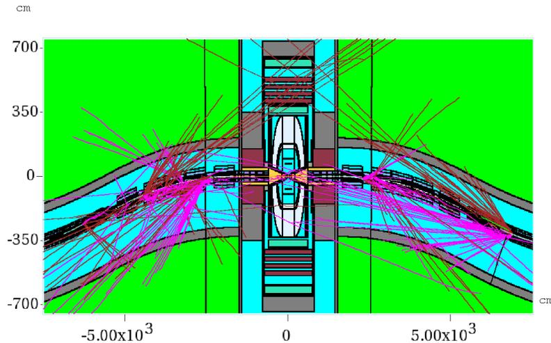
Figure 1: A MARS15 model of the IR and detector with particle tracks  $> 1$  GeV (mainly muons) for several forced decays of both beams.
