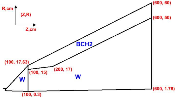
Figure 2: The MARS15 machine detector interface MDI (nozzle), 1/2 RZ view (W - tungsten, BCH2 - borated polyethylene).
