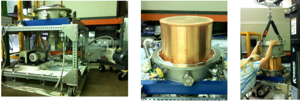
Fig. 4 (a) Dewar, vacuum pump, cryocooler, and compressor (b) Copper heat intercept shield (c) Closing the dewar
