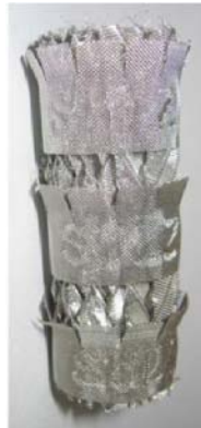
Figure 5. Custom packing material in the distillation column.
