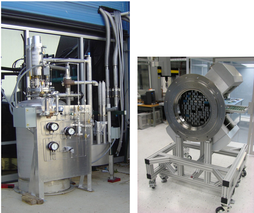
Figure 5. Left: Liquid nitrogen vessel and valve box for use at CTIO. Right: Imager Vessel
