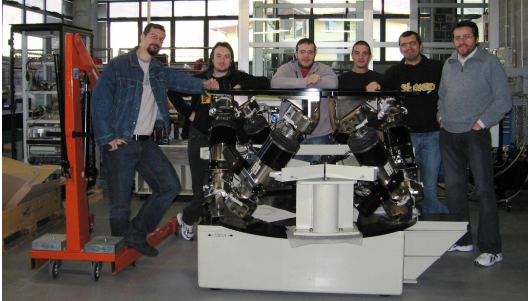
Figure 11 the assembled hexapod at ADS International, Valmadrera, Italy. The fixed flange is on the bottom. The assembly fixture is also shown.
