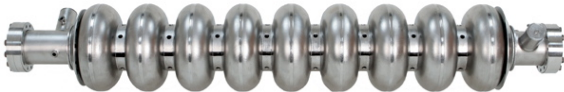
FIGURE 2. A photo of a 1.3 GHz, 9-cell, niobium SRF cavity. Stiffening rings are seen (with hole for helium penetration) between cells. This niobium structure is externally cooled by and pressurized by the helium bath.
