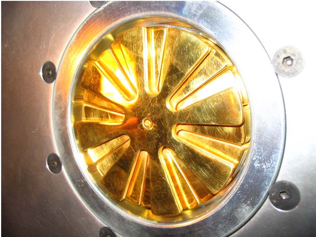
Figure 3.1 Photo of the 4" GVM installed in the Pelletron tank.
