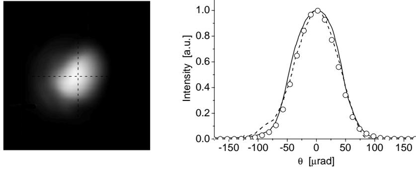
FIG. 3: Left: photon beam image on a Ce:YAG crystal averaged over many shots. Right: vertical (solid line) and horizontal (dashed line) slices of the image. Circles represent simulation results with the code FAST (40). The average energy in the radiation pulse is  $40 \mu\text{J}$ . The radiation wavelength is  $13.7 \text{ nm}$ .
