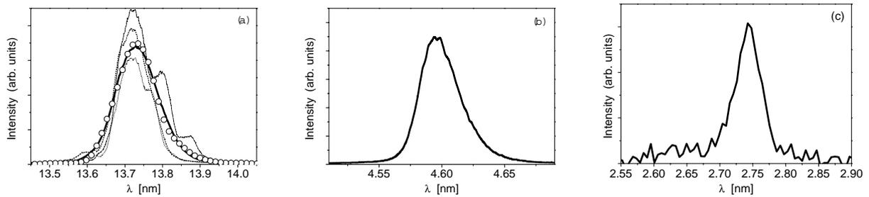
FIG. 5: EUV spectra of the fundamental (left), 3rd harmonic (center) and 5th harmonic (right) contributions to the FEL output. Bold lines show averaged spectra (mean value of 300 shots), and thin lines show single-shot spectra. Circles on the left plot represent averaged spectra simulated with the code FAST (40). The average energy in the FEL pulse is  $40 \mu\text{J}$ .
