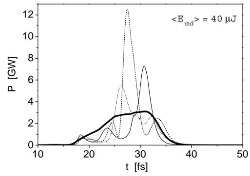
FIG. 6: The temporal structure of the radiation pulse, for an average energy of  $40 \mu\text{J}$ , predicted by the code FAST (40) using experimentally determined radiation properties. The radiation wavelength is  $13.7 \text{ nm}$ . The bold line shows the envelope while the thin lines are single shots.
