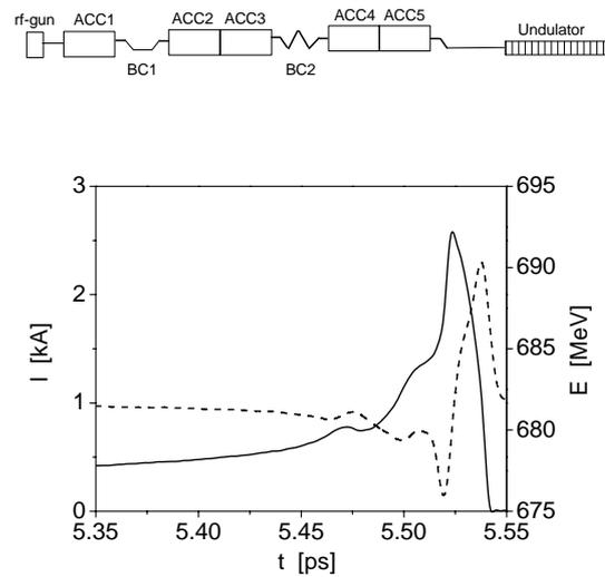
FIG. 2: Top: Schematic layout of the FLASH facility. Abbreviations ACC and BC stand for accelerating module and bunch compressor, respectively. Bottom: current  $I$  (solid line) and mean energy  $E$  (dashed line) along the electron bunch at the undulator entrance (simulations results). Bunch head is at the right side.
