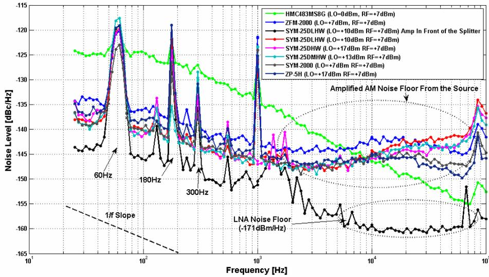
Figure 4: Measurements of Residual Phase Noise in the receiver's front end with various commercially available mixers.
