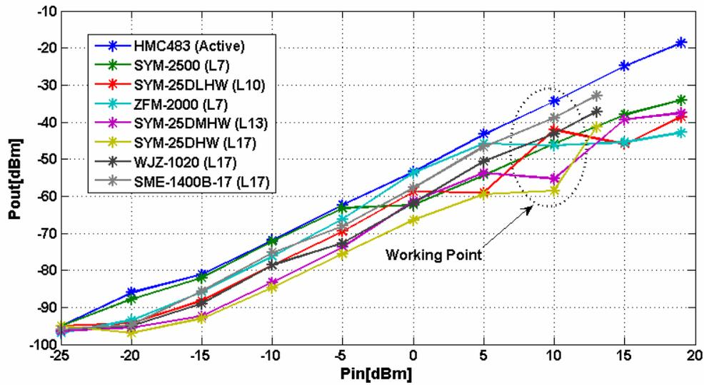
Figure 6: Power of the second harmonic at the IF port as function of input power on the RF port for various mixers.
