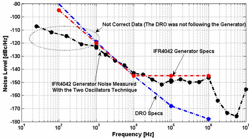
Figure 3: The generator noise in dBc/Hz (black) compared to the manufacturer's values (red) and compared to the specified phase noise values of the dielectric resonator oscillator (DRO [14]) in blue. The DRO was used for measuring the generator noise using the phase noise analyzer from Wenzel Associates, Inc. [15].
