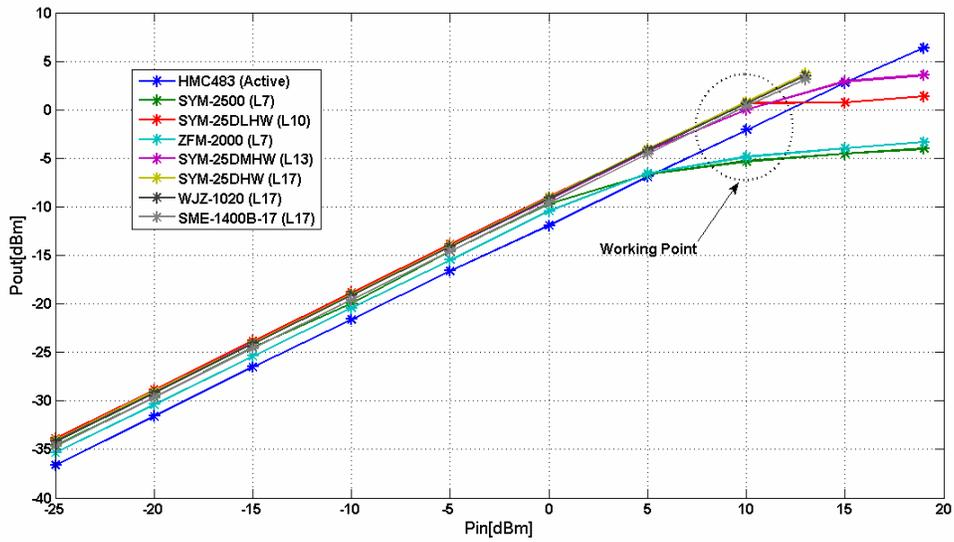
Figure 5: Output power of the carrier as function of input power on the RF port for various mixers.
