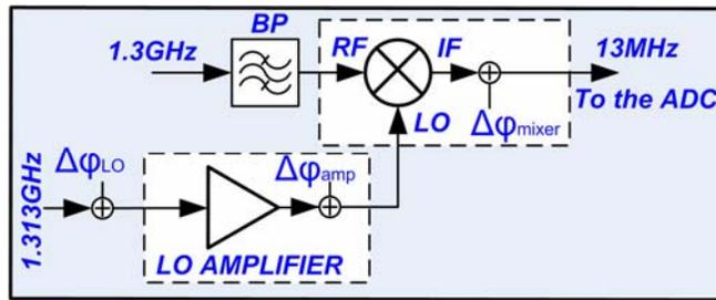
Figure 1: Block diagram of the receiver's analog front-end used in high energy physics for control of electromagnetic fields in superconducting RF cavities.
