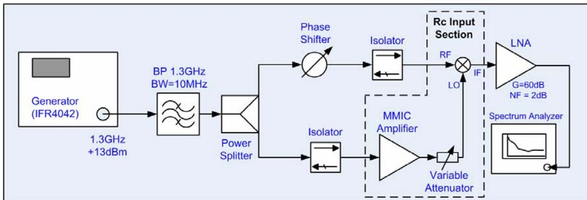
Figure 2: Residual phase noise measurements test setup.
