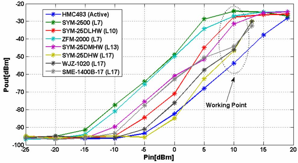
Figure 7: Power of the third harmonic at the IF port as function of input power on the RF port for various mixers.
