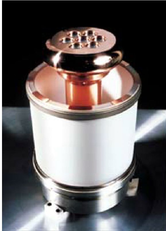
Figure 14.5: Cathode of Thompson multi-beam klystron.
