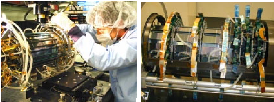
Fig. 6. (left) one of three CDF barrel sections under construction; (right) south half of the DØ silicon detector completed.
