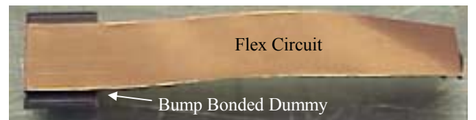
Figure 9: Dummy Bump Bond Structure
