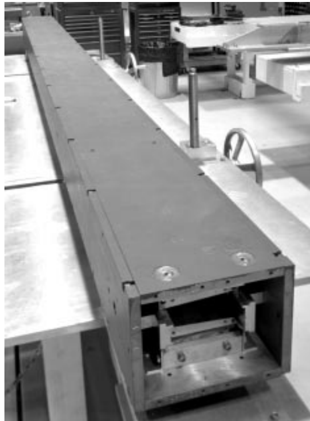
Figure 5: View of gradient magnet on assembly table.
