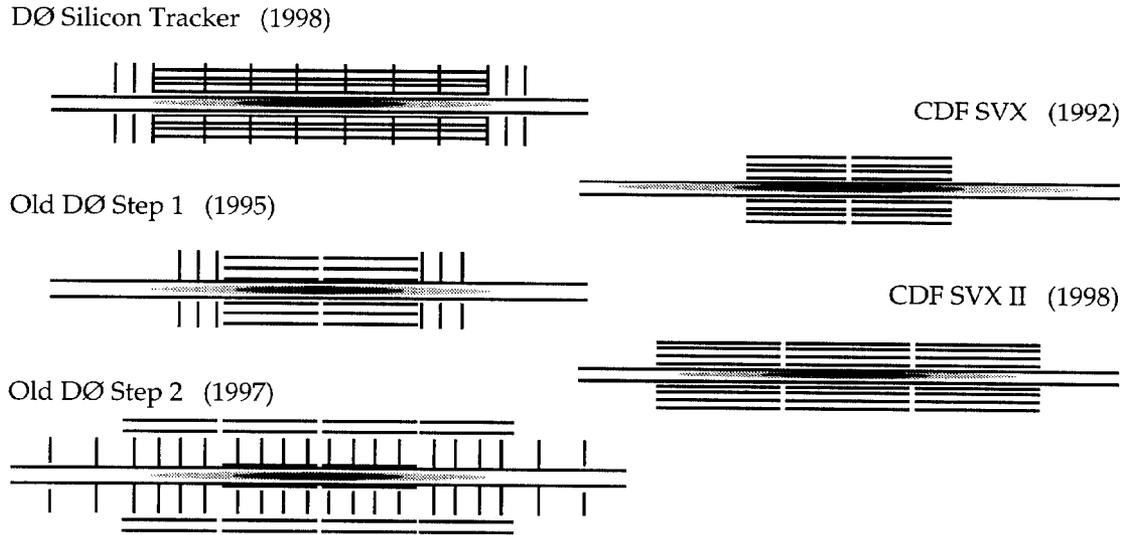
Fig.1 A comparison of silicon tracker designs at the Tevatron collider.
