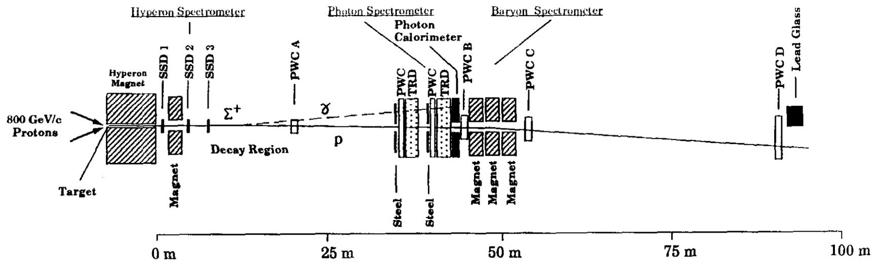
FIGURE 1. Plan view of the apparatus in the Fermilab Proton Center charged hyperon beam.
